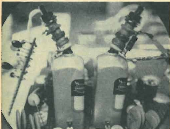
Fig. 10. Pickup coil (left) and injection coil are stuck into i.f. transformers to which these inductive probes are coupled.
